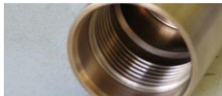
Ground rod threading
