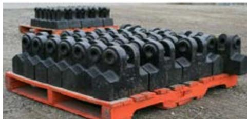
Titanium Carbide Hammers
